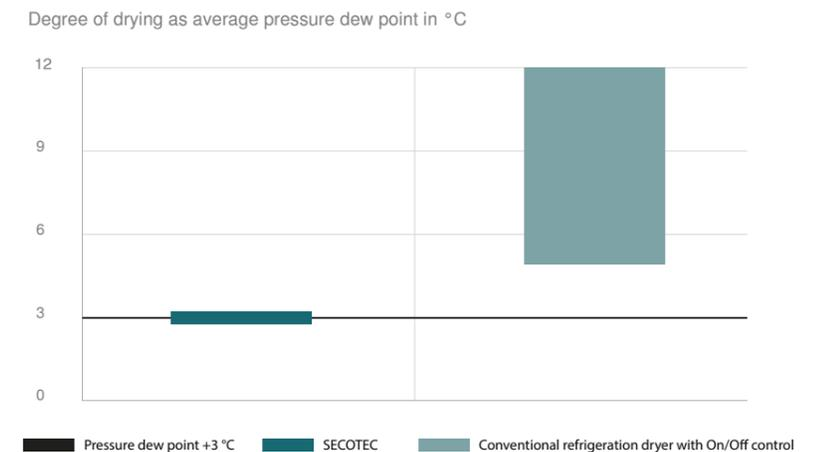
SECOTEC refrigeration dryers, on the other hand, ensure material-friendly operation thanks to their high thermal mass storage capacity. Once the thermal mass has been charged, the refrigerant compressor and fan motor can remain switched off for much longer with no impact on pressure dew point stability.
